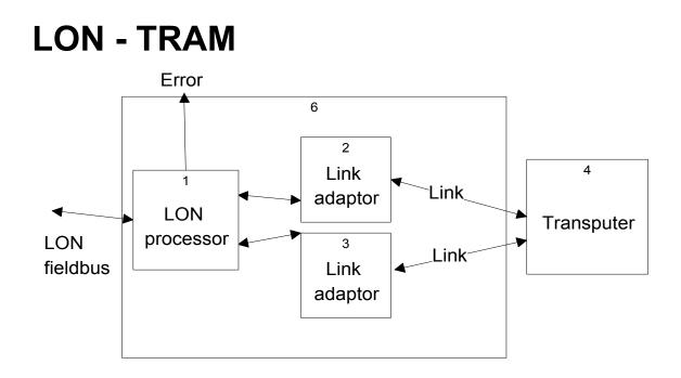
Neuron processor at 5Mhz, LON speed 78 kbit/Sec. Link to link speed:
