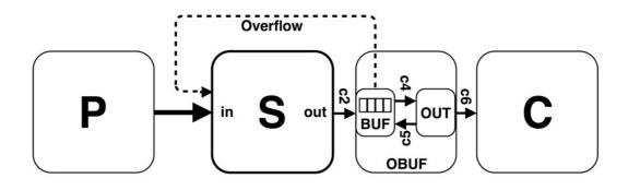
Figure 1. Example of an overflow buffer (OBUF)
